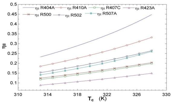
Figure 10: Variation of Exergetic efficiency with Condenser temperatures  $(T_c)$
