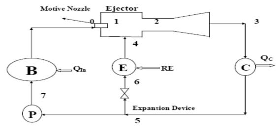
E: Evaporator; B: Boiler; C: Condenser; P: Pump
