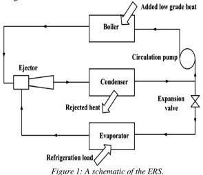
The inter-relation between the different parts can be expressed by the fig. 1. Boiler used low grade energy to produce vapours to be expanded inside the ejector. Without a compressor can this system perform saving high grade energy and cost.
