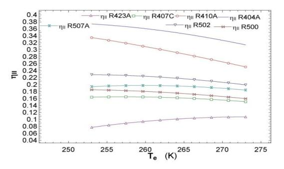
Figure 13: Variation of Exergetic efficiency with evaporator temperatures.
