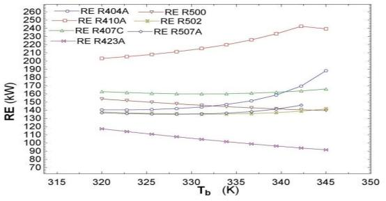
Figure 5: Variation of Refrigeration effect (RE) with boiling temperature  $(T_b)$
