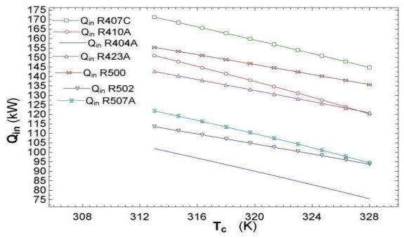
Figure 9: Variation of heat input required with Condenser temperatures. $(T_c)$
