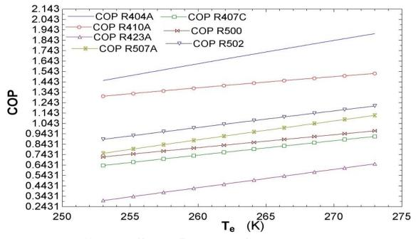
Figure 11: Variation of first Law Efficiency (COP) with evaporator temperatures ( $T_e$ )
