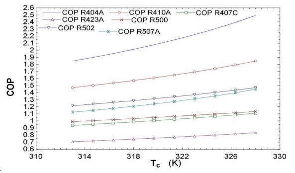
Figure 8: Variation of first Law Efficiency (COP) with Condenser operating temperatures.  $(T_c)$
