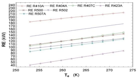
Figure 12: Variation refrigeration effect with evaporator temperatures  $(T_e)$
