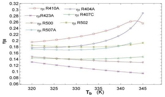
Figure 6: Variation of Second (Exergetic efficiency) with boiler temperature  $(T_b)$
