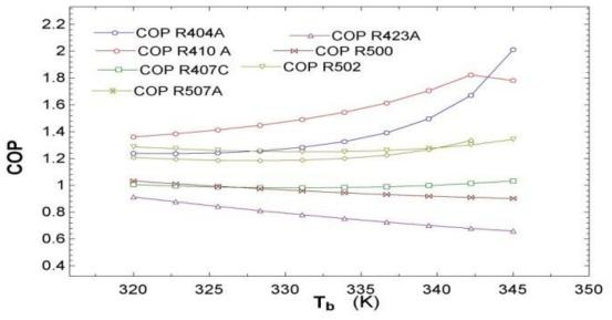
Figure 4: Variation of first law efficiency (COP) with boiler temperature  $(T_b)$
