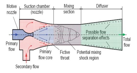
Figure 2: Schematic of a typical two-phase ejector design [10]
