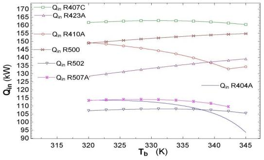
Figure 7: Variation of heat supplied to the boiler with boiler temperature  $(T_b)$
